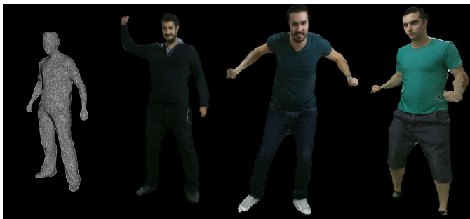
Fig. 2. 3D reconstructions produced by the studied 3D media tele-immersive pipeline. On the leftmost the pure geometry output is shown, while on its right the remaining three 3D reconstructions depict fully textured outputs from viewpoints other than those used to produce them.
