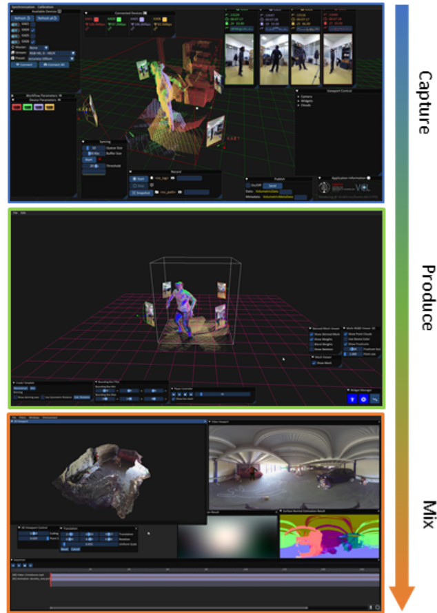
Fig. 1. Screenshots of the three cascaded XR360 toolkit. Top: The volumetric capture tool with a live point cloud visualization of the actor in the capturing space. Middle: The performance capture application while tracking the movement of the actor. Bottom: The 360° Fusion tool, visualizing a 360° scene’s estimated point cloud, surface normal and illumination.
