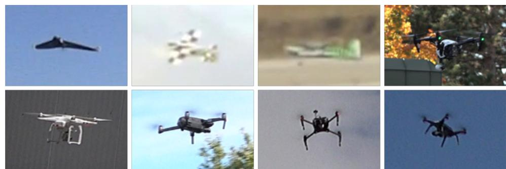
**Figure 1.** Examples of drone types present in the dataset, i.e., Parrot Disco, 2 custom fix wing drones, DJI Inspire, DJI Phantom, DJI Mavic, DJI Matrice and 3DR Solo Robotics.
