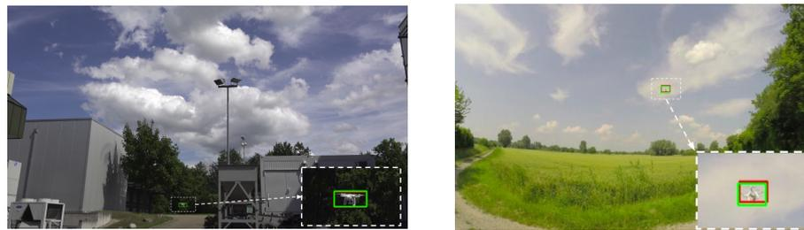
**Figure 18.** Alexis team approach based on YOLOv3 [39] is able to detect small drones in high resolution images by using an image tiling strategy. Here are some examples of successful detections made by their approach (green: predictions, red: ground-truths).
